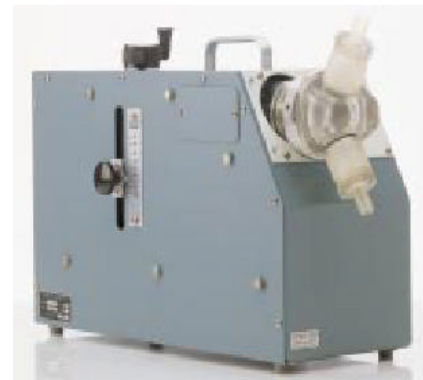
Figure 3: Harvard Pulsatile Pump. The pulsatile pumping mechanism consists of a piston actuator and ball check valves. These components aim at reproducing physiological flow conditions.
