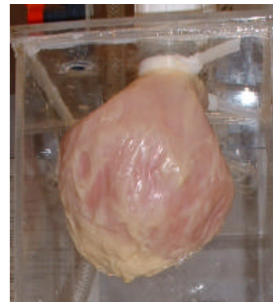
Figure 8: Latex Balloon. This latex balloon represents one of our initial ventricle prototypes
