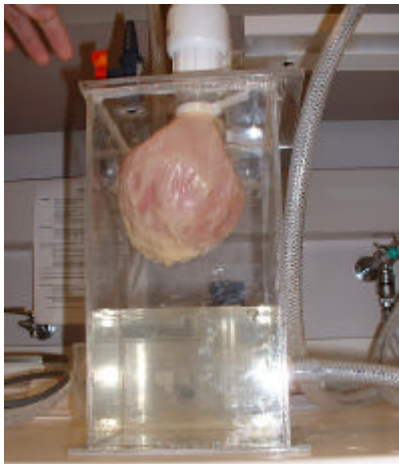
Figure 6: Chamber Prototype. This clear, acrylic chamber encloses the deformable ventricle model and is pressurized during flow.
