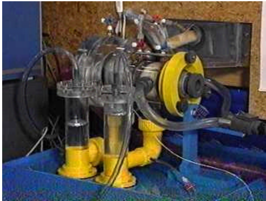
Figure 4: Pulse Duplicator System. Designed at Ghent University in Belgium, this model of the left heart incorporates a pressurized air system to regulate and monitor flow through the mitral and aortic valves.
