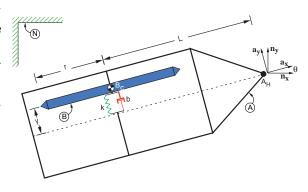
where v measures the speed of the hitch-point in the  $\mathbf{n}_{x}$  direction.
