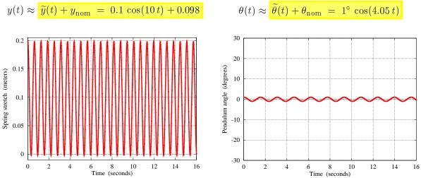
(i) (6 pts.) The computer solution for y(t) and  $\theta(t)$  to the original nonlinear ODEs for  $0 \le t \le 16$  sec are plotted below. Comment on the similarities and differences between the plots you produced with the ones below. Give a reason for the similarities and differences.
