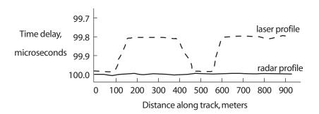
A clever student realizes that the laser is reflected from the tops of the trees while the radar signal penetrates to the forest surface, resulting in a greater time delay.
