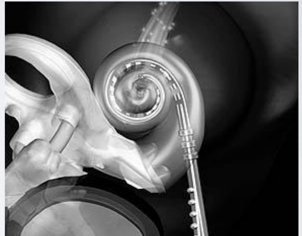
Visualization of a cochlear implant with an electrode array
