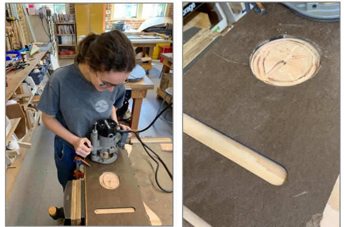
Figure 28. Olivia practicing making indentations for Abby's water bottle and pencils using a hand router.
