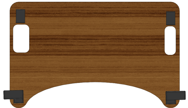
CAD model of the bottom view (underneath) of laptray with clip mechanism and front supports
