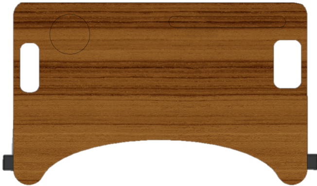
CAD model of top view of laptray with clip mechanism and visible water bottle and pencil indentations
