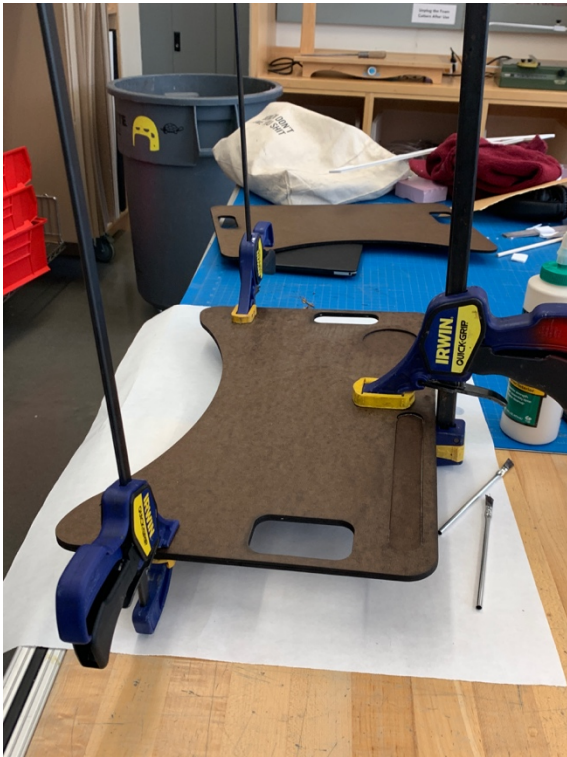
Fabrication of our layered 3/8inch Duron prototype with indentations for Abby's water bottle and pencils.
