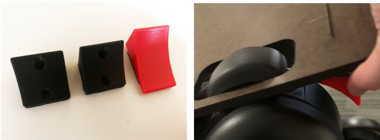
3D printed prototypes of the front supports of the laptray designed to increase the overall stability of the laptray.
