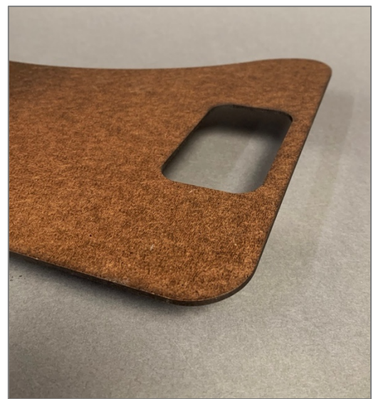
Figure 11c. Close up of laser-cut controller slot
