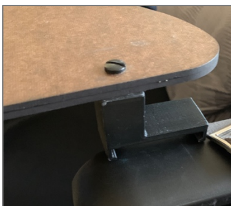
Figure 26. Clip contact with armchair obstructing the inclined mode
