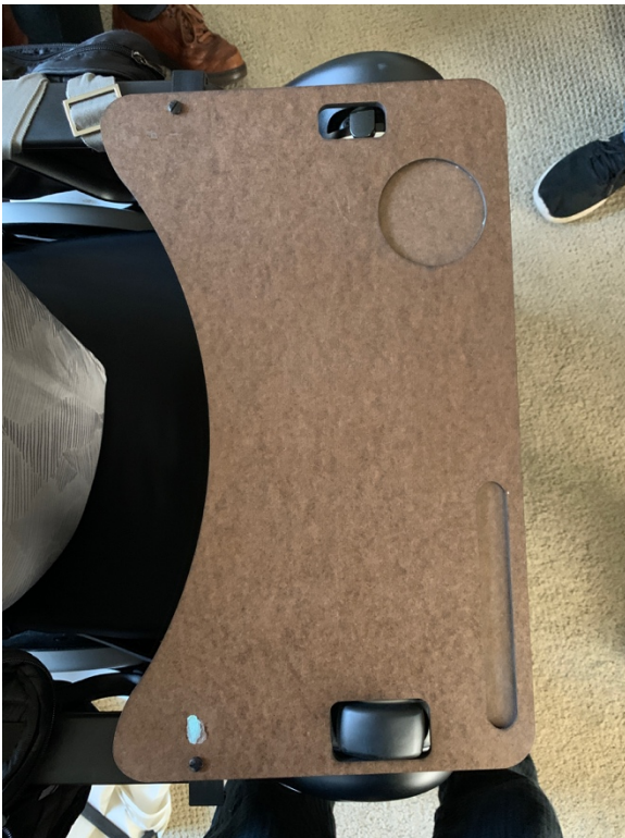
Team Laprador's seventh and final Duron prototype with the correct dimensions for the controller slots and indentations
