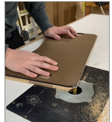
Figure 18. Jinho using the table router and Duron guide to shape the laptray
