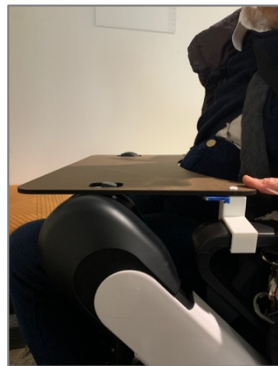
Figure 20a. Rotating clip positioned in the flat setting, with Abby exhibiting the laptray in this setting
