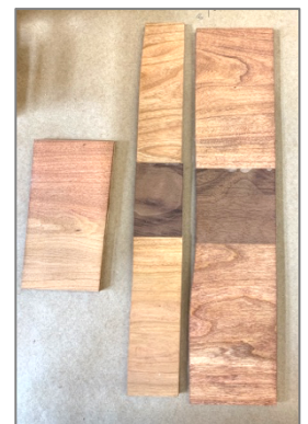
Figure 24. Stain testing between cherry (center) and maple (right) wood stains
