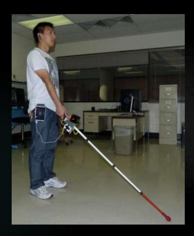
A co-robotic cane developed at the University of Arkansas at Little Rock promises to make life easier for blind people to navigate. The cameras detect obstacles in the user's path and provide audio feedback to facilitate safe travel. In addition, the cane provides guidance via a rolling tip that points in the proper direction. Link
