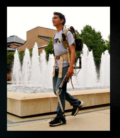
Student team STARX (STrength Augmenting Robotic eXoskeletons) completed its second year, focused on making practical powered exoskeletons that increase the effective strength of the user. This year, they built a new load-bearing exoskeleton called the Lexo. In its finished state, this device will transfer a load of up to 100 lbs off of the user and into the ground so they do not feel the weight. Link
