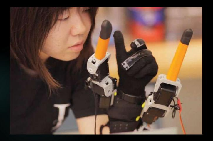
This MIT project added two large fingers to a glove. It lets users do things like hold an object with a couple of fingers while using the others to perform another job such as adding salt to a cup of liquid or opening the top of a jar. <u>Link</u>
