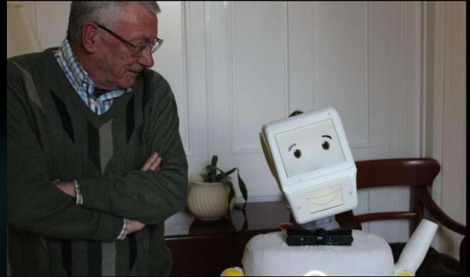
Stevie can perform some of its jobs autonomously, for example reminding users to take medication. It can also help users stay socially connected. For example, the screens in the head can facilitate a Skype call, eliminating the challenges many users face using telephones. Stevie can also regulate room temperatures and light levels, tasks that help to keep the occupant comfortable and reduce possible fall hazards. Link
