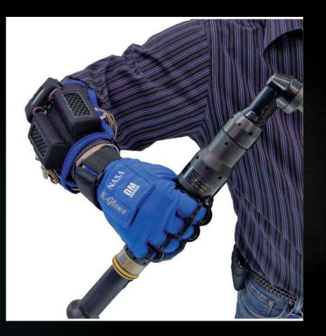
RoboGlove is essentially a wearable exoskeleton gripping tool. It addresses repetitive stress syndrome by reducing the amount of stress involved in an action or process.
