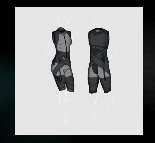
Superflex's elastic muscle technology, developed originally under a DARPA grant intended to help soldiers carry gear with less fatigue, looks like the marriage of a wetsuit and kinesio-tape. An onboard computer ensures that it flexes in concert with your real muscles, much like an electric bike that supplements your pedaling with its motor. Link
