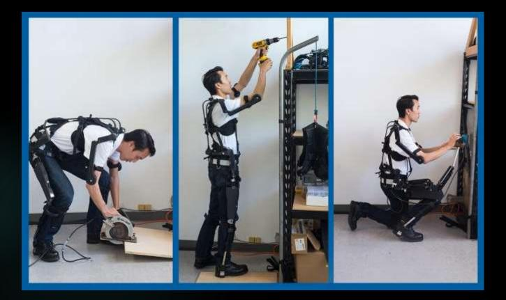
MAX (Modular Agile eXoskeleton) is a workplace exoskeleton in three modules that allows workers to complete shoulder, lower back and leg-intensive tasks with reduced injury risk. <u>Link</u>
