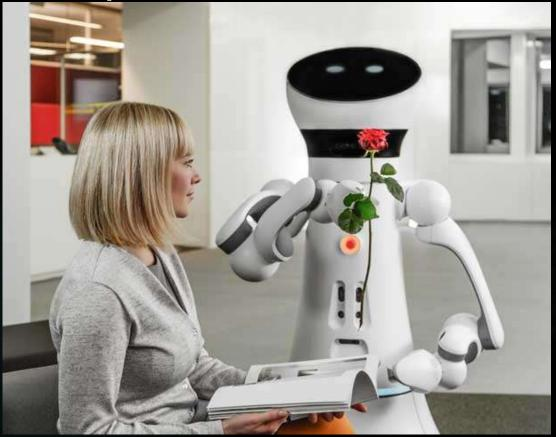
After two decades of refinement, the Care-O-bot 4 robot is constructed out of five modules: base, torso, arms, sensor ring, and head. Each one of these modules can be swapped out depending on what you want the robot to do (and what your budget is). Link
