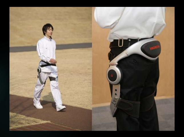
A variation of Honda's Walking Assist Device is being used in hospitals to assist in rehabilitation - is intended to help patients re-learn how to walk. Link
