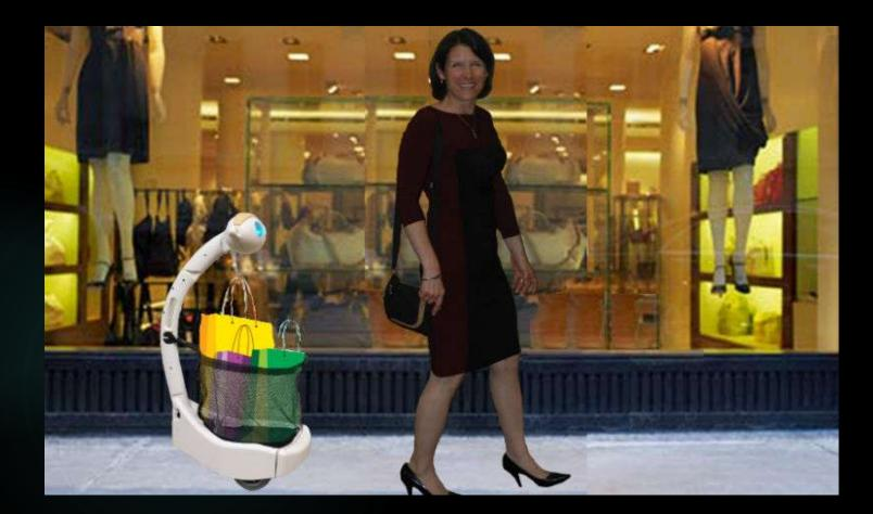
Budgee, the robot assistant, can carry 50 pounds and run up to 10 hours on a charge, and it has sensors on the front and side to avoid obstacles. Link
