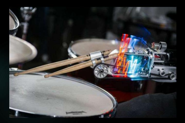
This robotic drumming prosthesis has motors that power two drumsticks. One is controlled by muscle sensors, the other is autonomous. Jason Barnes can now flex his muscles to send signals to a computer, which tightens or loosens his drumstick. Link
