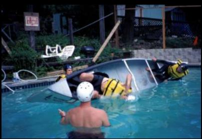
Test subjects are coached during the water portion of the evaluation in which the subject finally gets dumped on the count of three to verify safe egress from the canoe. At least one water safety expert is always on hand for this part of the evaluation.
