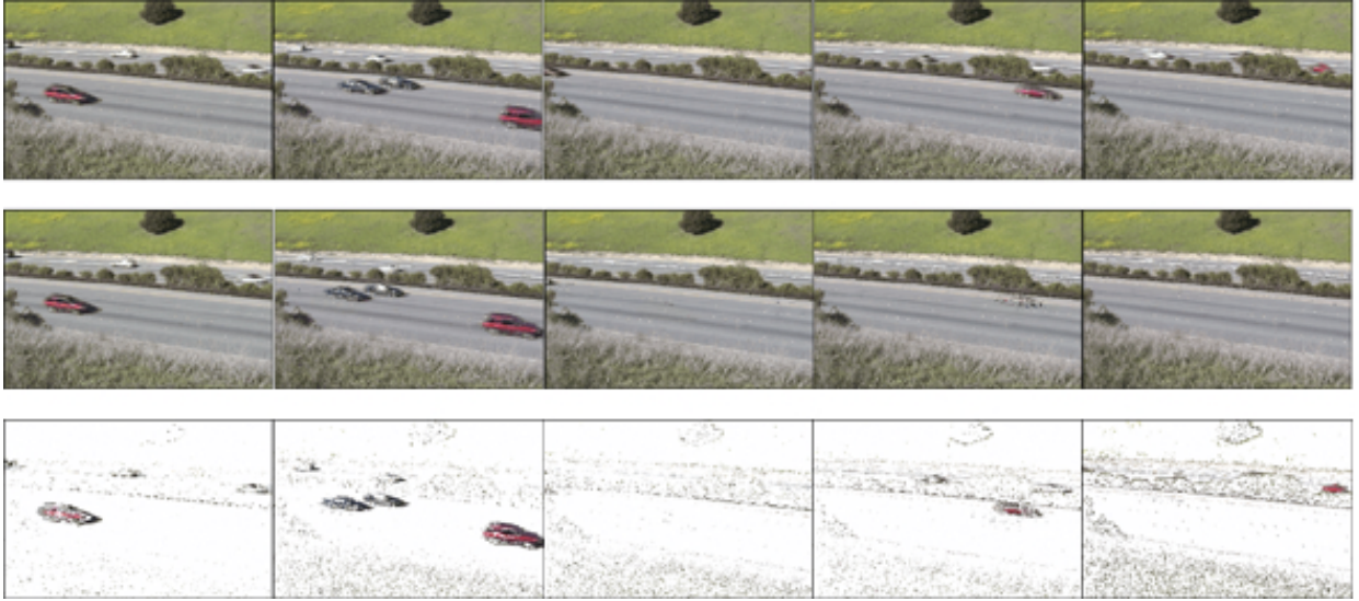
Fig. 3. Segmentation of freeway.avi. Left to right: frames 2, 26,52,78,104. Top to bottom: Original, Background, Foreground. This sequence has less global motion, so the extracted foreground appear to be clearer than those of the previous sequences.
