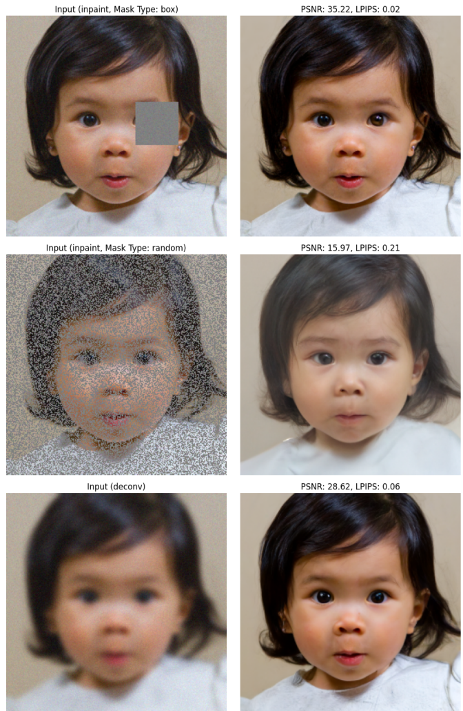
Fig. 6. Results of DPS on inpainting and deconvolution problems.
