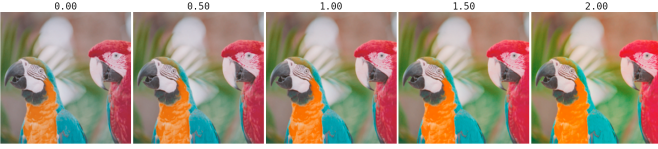
Fig. 4: The Effect of DIR Couplers: As the amount of DIR couplers increases, the resulting image becomes more saturated.
