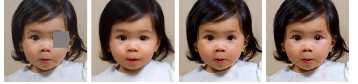
Fig. 7. Input image (a) followed by DPS output on an inpainting task with scale values (b) 0.1, (c) 0.3 and (d) 1.0. Too low a scale parameter reduces the effectiveness of inpainting. Higher scale factors (0.3 and 1.0) show good similarity to the input image.
