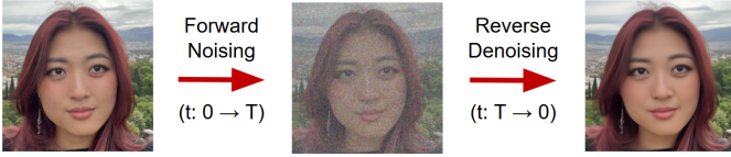
Fig. 2. The DDPM forward diffusion process gradually corrupts a clean image by adding Gaussian noise over timesteps t = 0 \rightarrow T . A learned reverse process then iteratively denoises the image to recover a realistic sample as t \rightarrow 0 .
