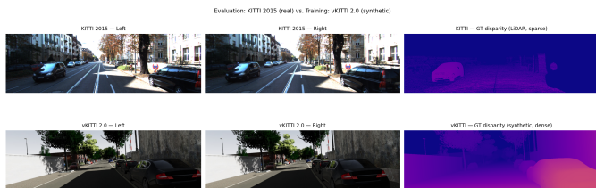
Fig. 3. Top: KITTI 2015 stereo pair with sparse LiDAR ground truth (evaluation). Bottom: vKITTI 2.0 stereo pair with dense synthetic ground truth (training). Note the density difference: KITTI GT is sparse (LiDAR points only) while vKITTI GT is fully dense, enabling richer supervision.
