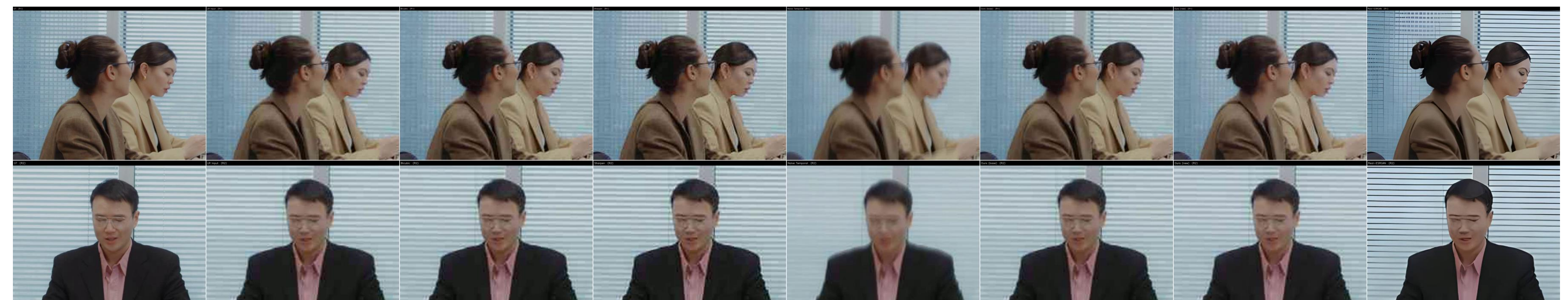
L-R: 4k Ground Truth, Low Resolution Input, Bicubic Upscaling, Whole Frame Sharpening, Naive Temporal Accumulation, Ours (No Sharpening), Ours (Sharpening), Real-ESRGAN
