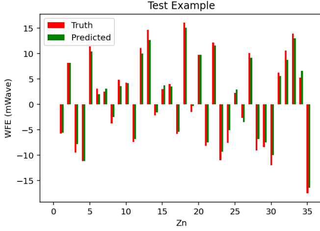
Fig. 8. One Test Example of Linear Regression - Zernike Coefficients
