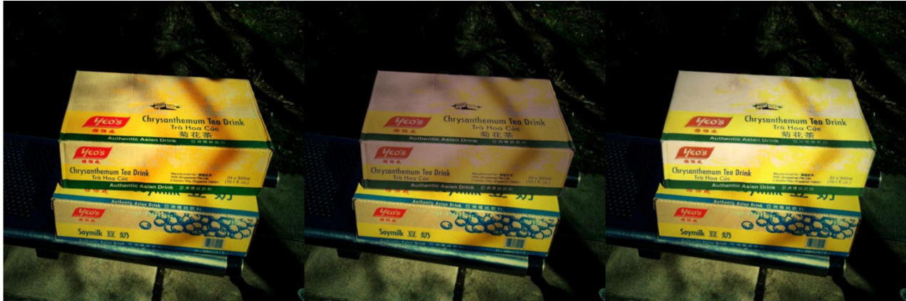
Fig. 1. A group of ground-truth real image (left), corresponding backward adjusted synthesized image (middle), and the harmonized image processed by Intrinsic Compositing algorithm (right). As can be observed from the images, although the algorithm works pretty well in retrieving the overall color and shading of the composite image, it still needs to be proved under harsh lightening. For example, the shadow becomes less obvious and the lightening contrast is lower when compared to ground-truth image. The processed image also lose resolutions in minor details, like the words on the box
