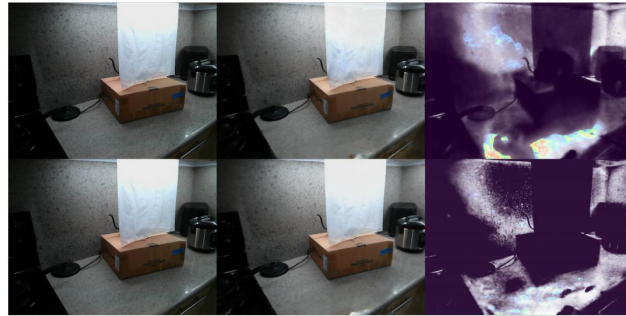
Fig. 5. Indoor scene of a hot kettle placed behind a sheet that is opaque in visible domain but transparent in thermal domain with our model (top) and RGB baseline model (bottom) - columns from left: ground truth, reconstructed RGB, RGB depth.
