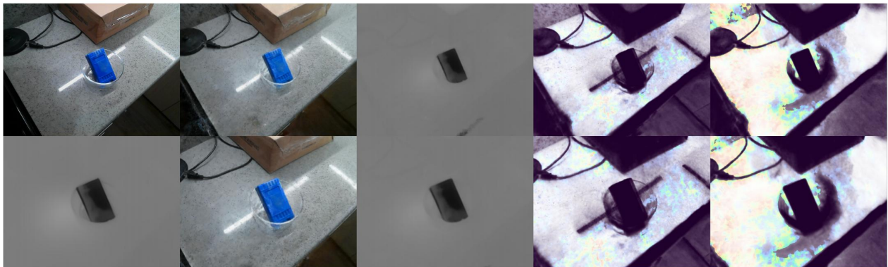
Fig. 3. Indoor scene of an ice pack in a bowl that is transparent in visible domain but opaque in thermal domain: columns from left: ground truth (RGB (top row), thermal (bottom row), reconstructed RGB, reconstructed thermal, RGB depth, thermal depth. Images obtained using Weights & Biases (wandb) which displays only either of the ground truths in the first column.
