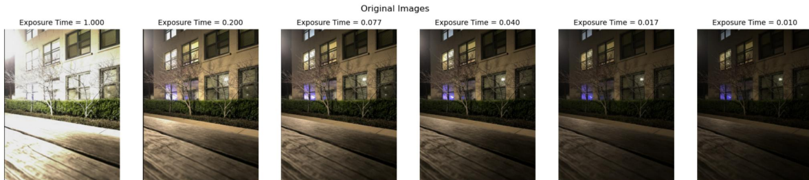
Fig. 2. Original set of images with the following exposure times: 1/1 s, 1/5s, 1/13 s, 1/25 s, 1/60 s, 1/100 s.
