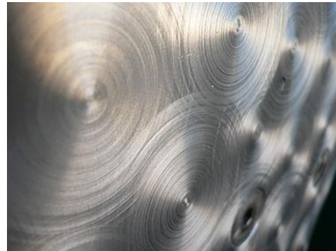
Figure 11. the difference in reflectivity on different direction for brushed metals.
