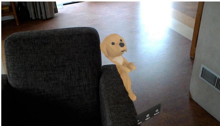
Fig. 1 - Microsoft Hololens Partially Occluded Dog [1]. Note how the dog is missing its neck and part of its body overlaps with the sofa indicative of a poor 3D mesh.
