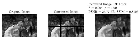
Figure 51. Original image, corrupted image with small square mask, and inpainted image of two basketball players with RF Prior.
