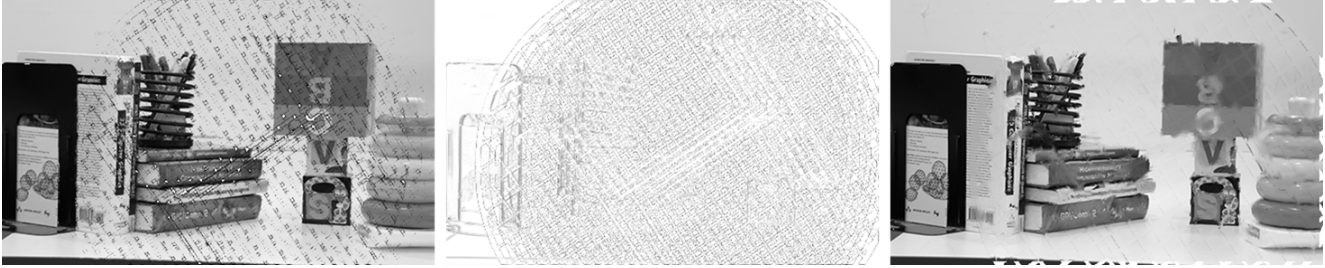
Figure 3: The median image is calculated by taking the median non-null pixel in each patch of the light field (left). The confidence value for each median pixel is also visualized (center). Using the median and confidence, we are able to synthesize the missing portions of the image (right).
