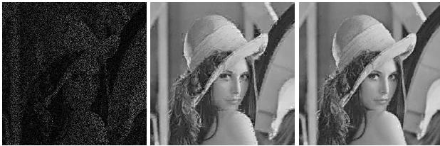
Figure 9. Left: Degraded image with 80% pixel loss, PSNR = 6.42dB Middle: Reconstruction using pre-defined DCT dictionary, PSNR = 24.27dB Right: reconstruction using KSVD learned dictionary, PSNR = 26.75dB
