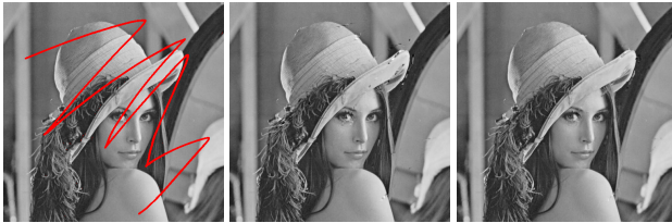
Figure 8. Left: Scratch degraded image, PSNR = 19.09dB Middle: Reconstruction using pre-defined DCT dictionary, PSNR = 33.68dB Right: reconstruction using KSVD learned dictionary, PSNR = 35.94dB
