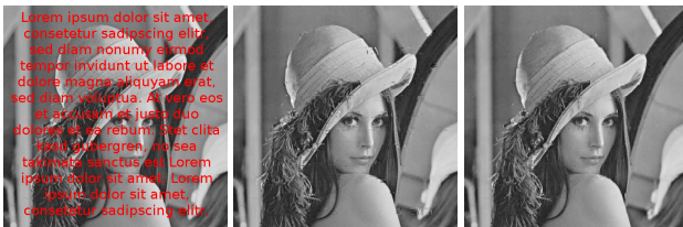
Figure 7. Left: Text degraded image, PSNR = 14.03dB Middle: Reconstruction using pre-defined DCT dictionary, PSNR = 30.9dB Right: reconstruction using KSVD learned dictionary, PSNR = 33.09dB
