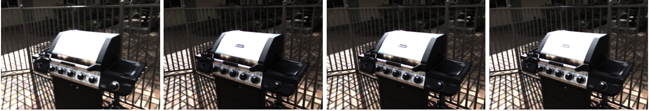
Figure 3. Comparison of Glare Reduction Based on Percentage of Rays Used as Outliers [L to R: Original Image (no glare reduction); 10% Rays Used; 25% Rays Used; 50% Rays Used (all manipulated in RGB)]
