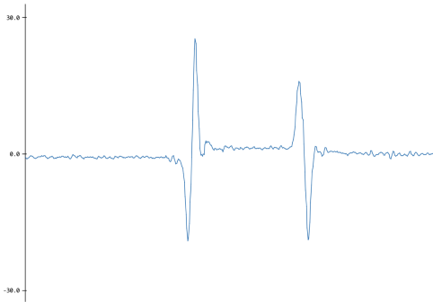
Figure 5: Component of linear acceleration along the Myo's forward direction. The first pair of peaks corresponds to a pull, and the second pair corresponds to a push.
