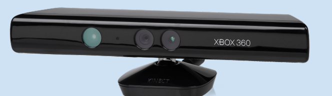
Kinect 360 Uses an RGB camera and infrared projection based depth sensor to track objects in its view
