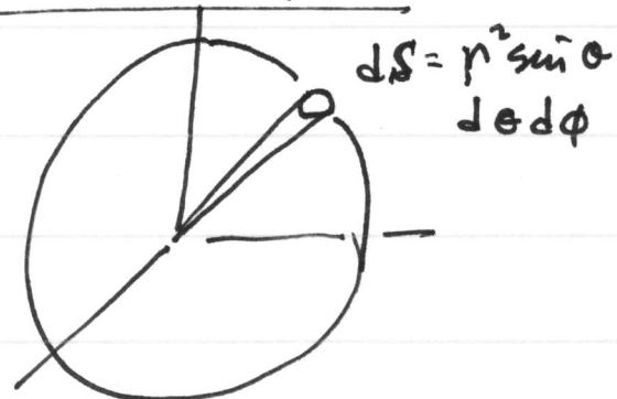
$$\text{Power} = \int_0^{2\pi} \int_0^{\pi} \frac{1}{8} \left( \frac{I \Delta \theta}{d} \right)^2 \frac{\sin^2 \theta}{r^2} \cdot r^2 \sin \theta d\theta d\phi$$
