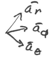
$$\bar{W} = \underbrace{\bar{E}_r H^*}_{\text{?}} = \bar{a}_r E_\theta H_\phi^* - \bar{a}_\theta E_r H_\phi^* + 0 \cdot \bar{a}_\phi$$
