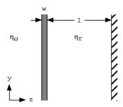
The screen is made of space cloth, which has the property that the resistance of a square is given by  $R = 377 \Omega = \eta_0$ . Remember that
