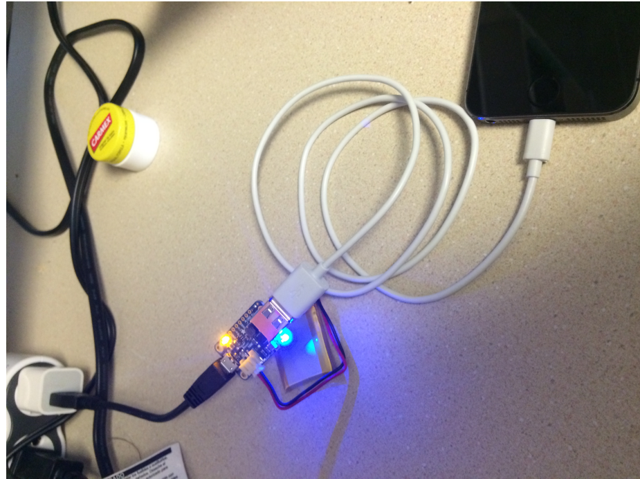
Figure H: Completed circuit from charging source to the circuit and then to the iPhone. Note that the circuit need not be plugged into the charging source to charge the phone.
