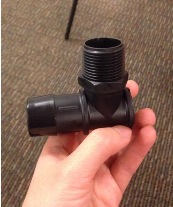
Figure 16: The resulting elbow pipe after cutting off the third edge
