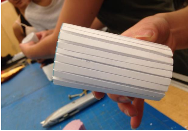
Figure 14: Foam core scored into a cylindrical shape
