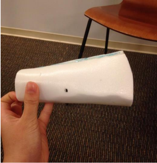
Figure 13: First mock up cone made of soft foam
