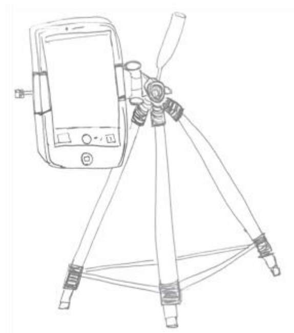
Figure 4. Sketch for the alternative design of the tripod with extendable legs
