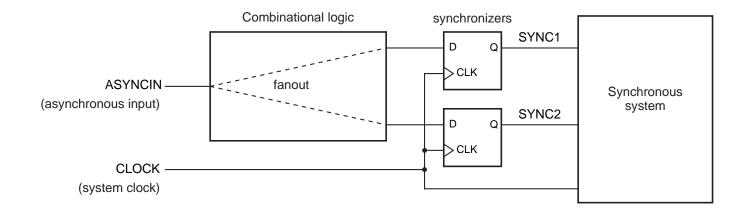
Solution: synchronize the variable for supplying it to combinational logic.
