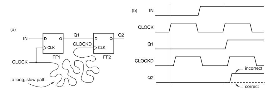
"Same" time means that difference between active edges should be small compared to hold time.
