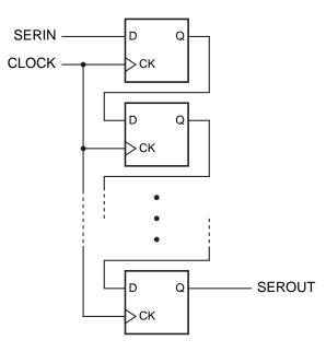
From DDPP Table 8-1, 74FCT273 has min  $t_{\rm ffpd} = 2$  and  $t_{\rm hold} = 1.5$ .
