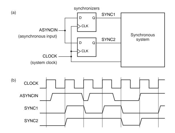
Sample an asynchronous signal at one place in your circuit. Otherwise, system might see inconsistent values of input.
