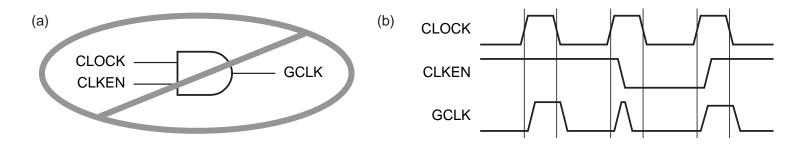
An "acceptable" way to gate the clock (reduces clock skew). Not in EE 121.
