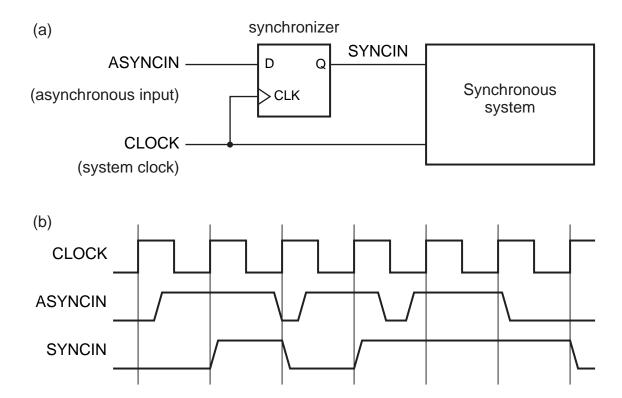
This works most of the time (failure rate proportional to system clock).
