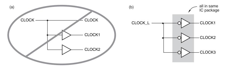
Master clock must be buffered through a tree so that slave clocks have same delay. (Done for you in Xilinx FPGAs.)
