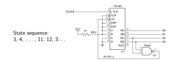
With one 3-input NAND gate, any period between 1 and 16 can be obtained. In fact, any low and high values can be specified.
