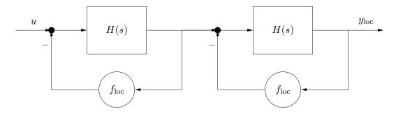
In both arrangements, the feedback consists of a positive gain (independent of s).
