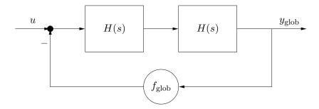
Local feedback. In this arrangement we use feedback around each amplifier, and then put the two closed-loop systems in cascade, as shown below. (To simplify things, we'll assume the two feedack gains are the same.)
