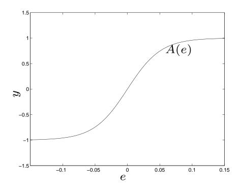
very common for amplifiers, transducers, etc. to be at least a bit nonlinear A is called the *nonlinear transfer characteristic* of the forward system (never to be confused with transfer function!)
