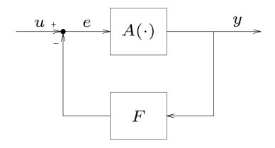
feedback system is described by y = A(e), e = u - Fy these are coupled *nonlinear* equations:
