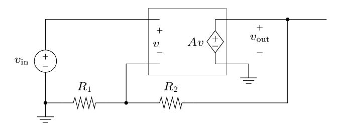
described by:  $v_{\text{out}} = Av$ ,  $v = v_{\text{in}} - (R_1/(R_1 + R_2))v_{\text{out}}$
