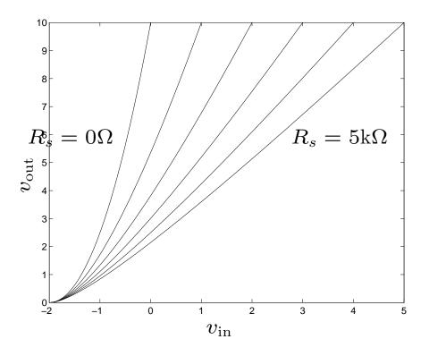
plot shows  $v_{\rm out}$  vs.  $v_{\rm in}$  for  $R_s=0,1,\ldots,5{\rm k}\Omega$  (corresponds to  $F=0,0.1,\ldots,0.5$ )
