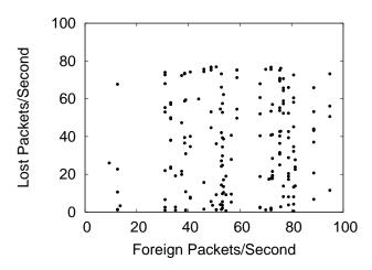
Figure 18: Each point indicates one host pair. The x-axis shows the number of foreign packets received per second by the receiver in that pair (same data as Table 1). The y-axis shows the number of 1500-byte packets lost per second at 1 Mbit/s. The data for the two axes are from experiments performed within a few minutes of each other. There is no obvious correlation.
