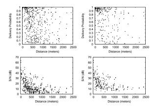
Figure 6: Scatter plots showing the relationship of distance versus delivery probability (top) and distance versus S/N (bottom). The left two graphs are for 1 Mbit/s, the right two graphs are for 11 Mbit/s. There is one point per pair of Roofnet nodes that are able to communicate at the given bit-rate.
