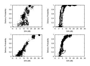
Figure 15: A scatter plot of average S/N vs average delivery probability at 1 Mbit/s. Each graph corresponds to a different receiver, each point shape corresponds to a different sender, and there is one point per one-second interval per sender.
