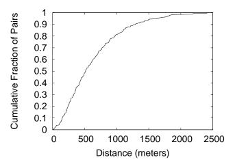
Figure 20: A CDF of the distance between all pairs of Roofnet nodes that have non-zero delivery probabilities for 1500-byte packets at 1 Mbit/s.
