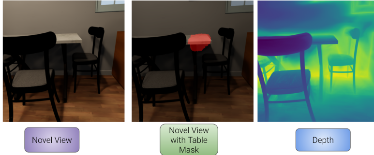
Figure 2: An example of the 3DGS pipeline – the novel view, the novel view with the table mask from CLIP-SEG, and the depth output from 3DGS.
