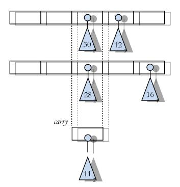
3. Merge the three (three!) order-2 trees! Leave one of the three alone (we'll leave the 11 in place, though it could have been any of the three) and merge the other two to produce an order-3 (with the smaller of 28 and 30 as the root).
