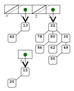
The carry now contributes to the merging at the order-1 level. The carry (with the 15 and the 20) and the original order-1 contribution (the one with the 13 and the 45) similarly merge to produce a NULL order-1 with an order-2 carry.
