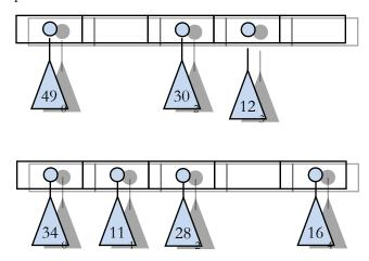
The triangles represent binomial trees respecting the heap ordering properties, and the subscripts represent their order. The numbers within the triangles are the root values—the smallest in the tree, and the blanks represent **NULL**. (We don't have space for the more elaborate pictures used to illustrate **enqueue**, so I'm going with more skeletal but I'm hoping equally helpful pictures.)
