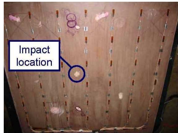
Fig. 7: Flat composite panel with 49 sensors.
