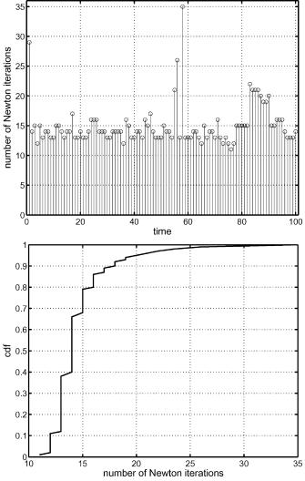
Fig. 2. Number of Newton iterations needed for reconvergence with Rayleigh fading channels. (*Top*) Number of Newton iterations for reconvergence during the first 100 time-steps. (*Bottom*) CDF of number of Newton iterations for reconvergence over 500 time-steps.
