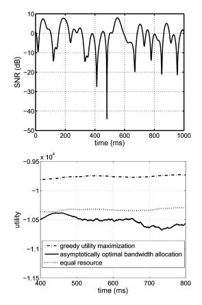
Fig. 3. Scheduling with memory and log utilities. (*Top*) Typical sample path of channel gain. (*Bottom*) Evolution of utility functions with time for three different scheduling policies.
