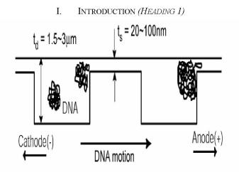
Figure 1. Nanofluidic DNA filter [2].
