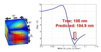
Figure 7. Optimization on 50-state parameterized reduced-order model predicts shape [9].
